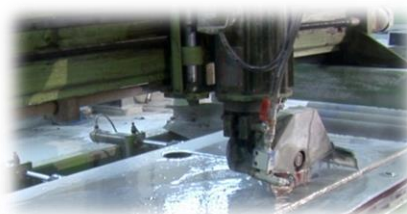
Cutting with bridge saw
