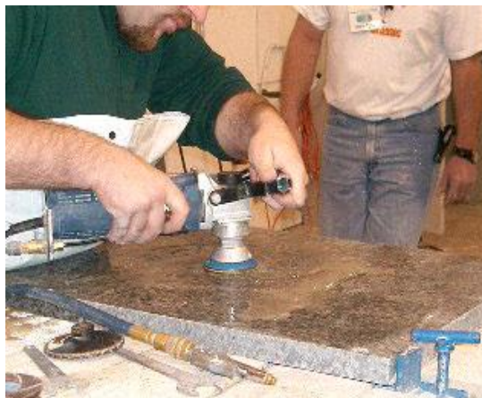
Scratch removing and polishing
