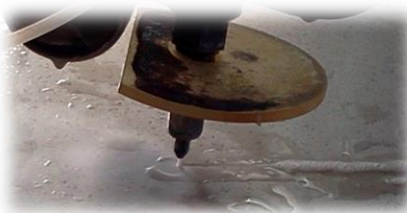
Cut-out by water jet
