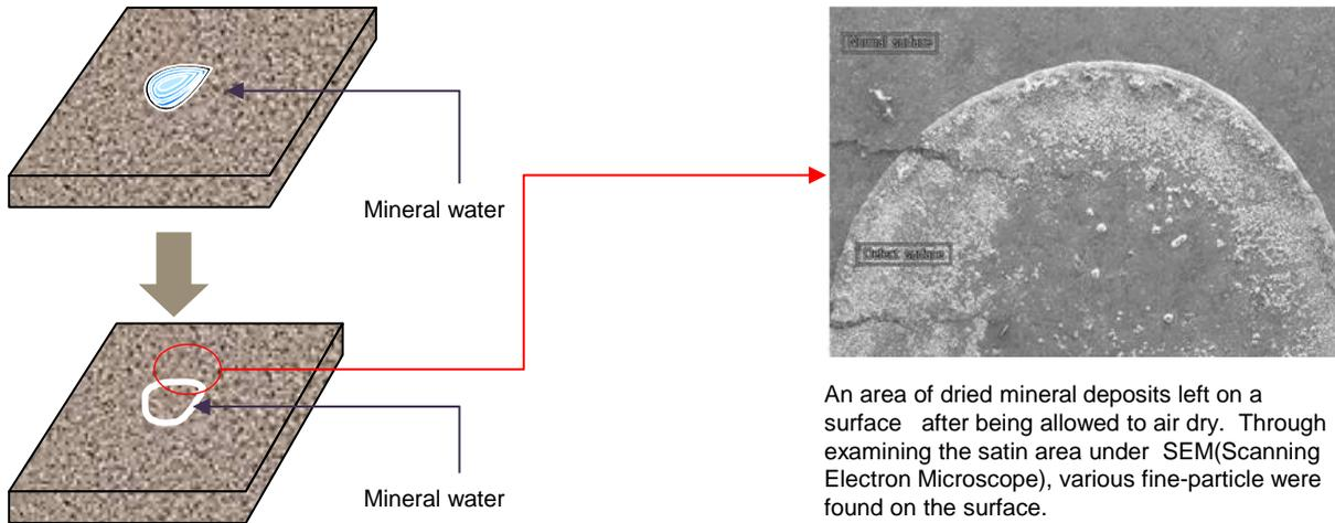
An area of dried mineral deposits left on a surface after being allowed to air dry. Through examining the satin area under SEM(Scanning Electron Microscope), various fine-particle were found on the surface.
